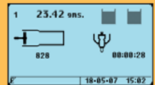
Operation screen displays current shot, material availability and pump ready indicators
